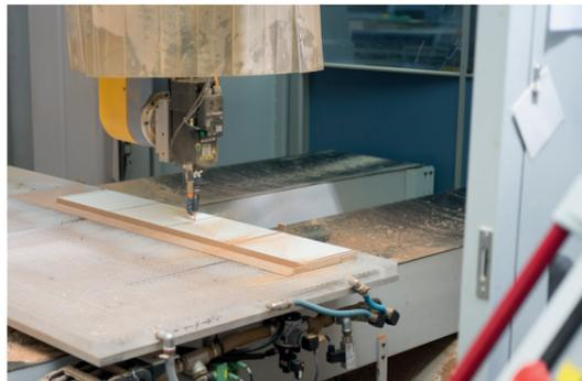
CNC Fräsen CNC milling Fraîsage CNC
